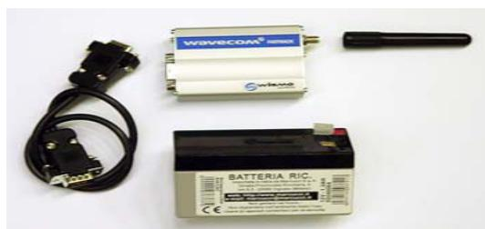
This bi-directional remote control and telemetry via GSM allows a check of both the complete system and of the parameters of each single transmitter
