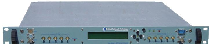
QPSK 70 MHz Modulator & Demodulator
