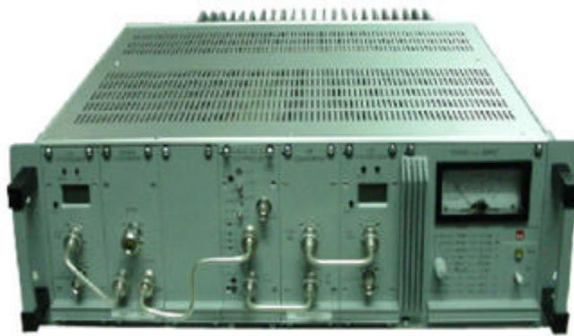
This kind of TV transposer, available in VHF and UHF, has been especially designed for low power repeater stations operating in difficult environments.
